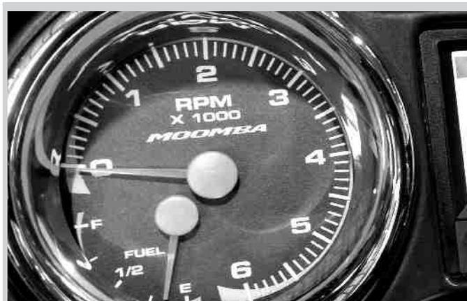
The tachometer registers the operating speed of the motor's shaft output and may be used as an alternative to speedometer if weight and water conditions permit.
