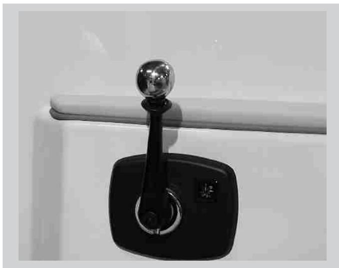
The throttle lever controls both the throttle and the transmission. The idle position (normally vertical) is the zero throttle position and the neutral position for the transmission. A safety ring (umbrella) keeps the lever from being accidentally moved to engage the transmission.
