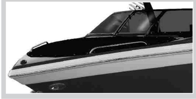
The optional tonneau cover is designed to snap over the bow of the boat. Its purpose is to minimize air flow into the cockpit area when the boat is in use and as a storage cover when used in combination with the optional cockpit cover.
