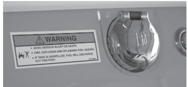
The fuel cap is located on the rear deck, 2-4 feet from the stern. To open, push the black tab located on the bottom side of the gas cap. When the black tab is pushed, the gas cap will hinge upward. To close, push the gas cap down. When the gas cap is completely closed a "click" sound should be heard. The audible "click" ensures that the gas cap is closed and sealed.
