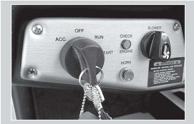
Located on the port side of the dashboard, the ignition switch has four positions. In the vertical position, the ignition is "OFF".
