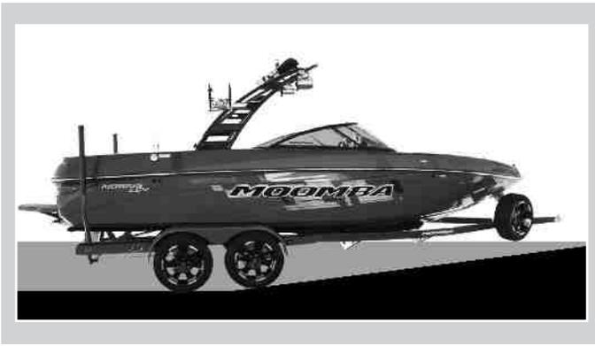
**NOTE: DO NOT attempt to use excessive power to free the boat from dry carpet runners. Power off of the trailer only when the boat has floated free.**
