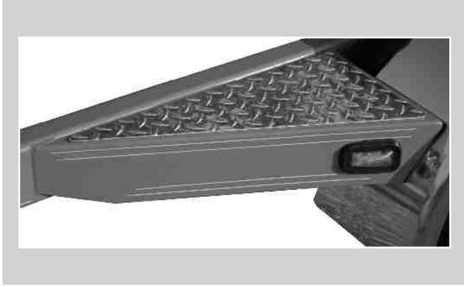
The optional aluminum step plate gives the trailer a durable long-lasting, nonskid surface on the trailer steps.
