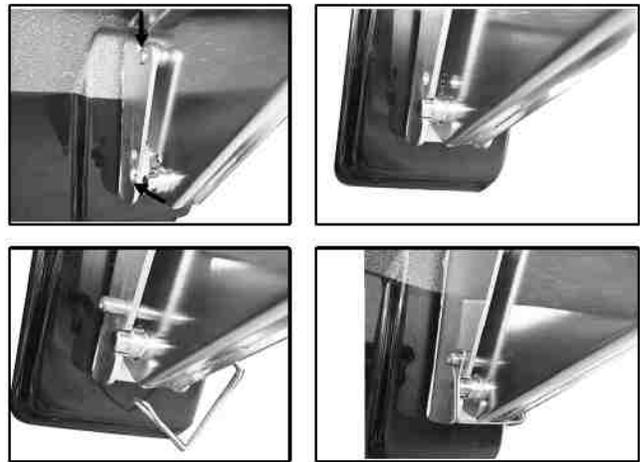
The ski platform is attached to the boat with detachable brackets. The platform may be removed from the boat by 1. Set platform on bracket. 2. Locate lower pin. 3. Locate locking pin through brackets. 4. Swing locking arm over end of pin.
