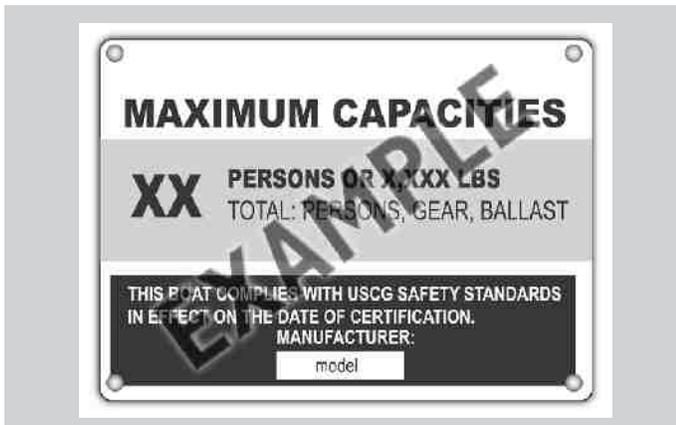
In compliance with United States Coast Guard Regulations, Moomba Boats meet or exceed all safety standards designed for recreational boats. To ensure safe handling and performance, each Moomba boat displays a maximum capacity sticker (see sample), stating the maximum passenger weight load allowable.
