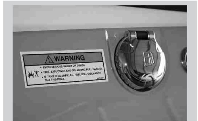
**NOTE: The gas cap is sealed by a rubber O-ring. Ensure the cap is clicked shut to properly seal.**
