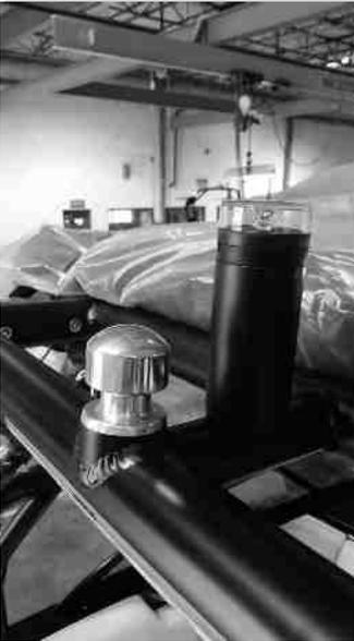
On boats equipped with factory installed towers, the 360° White Pole Light is mounted on the tower. To raise the light, pull the lever on the side of the light and then carefully raise the light to a vertical position. Always lower the light after use and before trailering to avoid hitting low overhangs.
