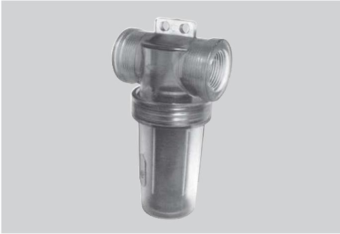
The optional ballast system also includes an in-line water strainer before the manifold. This strainer will keep debris out of the solenoid valve and should prevent the valve from getting clogged up and forced open. The strainer cover should be removed periodically and the filter screen cleaned to prevent debris buildup on the mesh screen. Be careful when removing the cover not to lose the O-ring used to seal the cover. Also, the strainer should be removed and drained during winterization.
