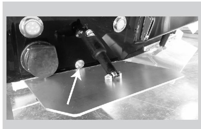
The rear drain plug is located at the back of the boat, near the bottom of the transom. It is extremely important that the drain plug is always checked before starting the engine. The drain plug should be secured in place using a wrench.
