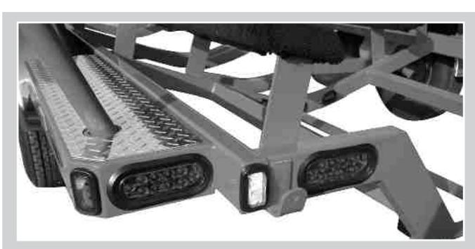
The standard LED lighting package replaces the traditional trailer lights with LED lights. The LED lights are brighter than the traditional lights.
