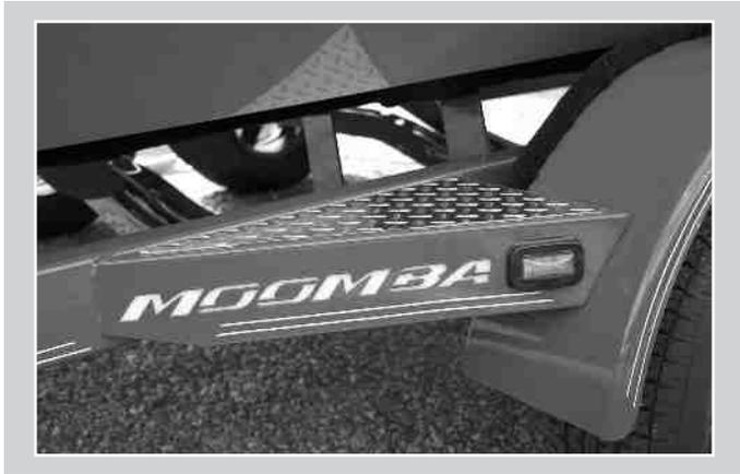
The optional laser cut steps are backlit so they illuminate when the trailer's running lights are illuminated.
