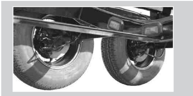
The standard second axle disk brakes give the trailer more stopping power.
