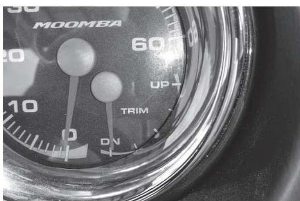
This switch controls the optional wakeplate. The gauge indicates the position of the wakeplate.
