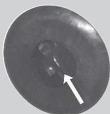
The speedometer pickup is located on the bottom of the hull. The pickup measures the speed of water passing the paddlewheel. Poor water conditions or foreign material may clog the pickup causing the speedometer to register incorrectly.
