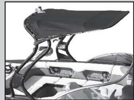
The bimini top is designed as a sunshade. Please see the mooring cover section for instructions on cleaning and caring for your bimini top. When opening and latching the straps to the eye hooks, twist the strap one to two times to prevent them from vibrating in the wind.
