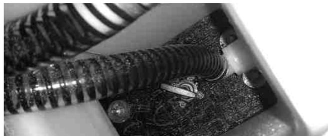
On V-drive models the center drain plug is accessed via the access cover in the center floor panel.
