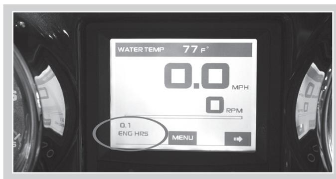
Engine hours should always be noted and documented so that required maintenance and lubrication changes may be performed at the proper intervals. The engine hour meter indicates the number of hours the engine has run.
