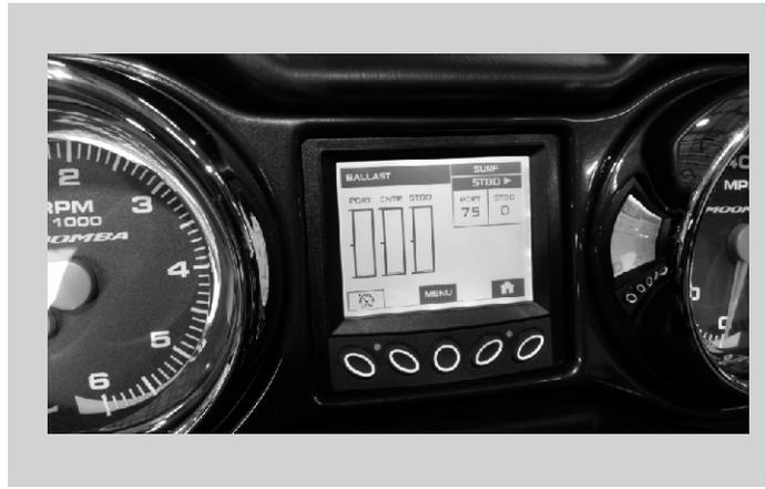
The Ballast System in your boat is electronically controlled and can be operated from the driver's seat. The manual switches for this three position system can be located to the right of the steering wheel.
