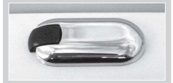
The pole light receptacle is located on the port side deck near the stern. To install the pole light, open the cover completely and with the plug correctly aligned, slide it into the socket until the electrical contacts are firmly in place.
