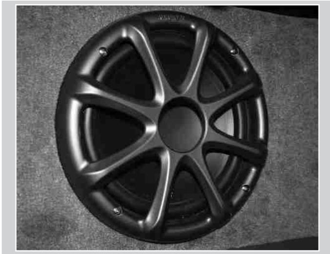
The optional sub-woofer is designed to increase the sound level of the bass notes. The optional amplifier powers the sub-woofer. The bass level can be adjusted on the amplifier. Please see stereo amplifier owner's manual for more information.
