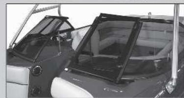
The moveable center windshield panel allows access to and from the bow area on some models. To open, turn safety latches to vertical and push. Carefully lay the hinged windshield panel back against the fixed side panel.
