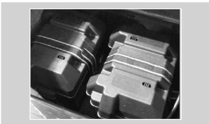
The battery box is mounted on the inside of the observer's seat storage compartment.
