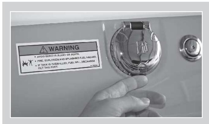
The fuel cap is located on the rear deck, 2-4 feet from the stern. To open, push black tab located on the bottom side of the gas cap. When the black tab is pushed, the gas cap will hinge upward.
