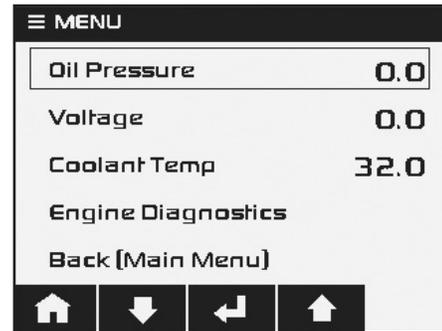
This screen displays the Oil Pressure, Voltage and Coolant Temperatures. The Engine Diagnostics link will display the following screen. Back (Main Menu) returns to the previous screen. Engine Diagnostics The Engine Diagnostics screen will appear as follows:
