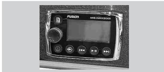
The optional transom mounted stereo remote allows the stereo to be controlled from the rear of the boat.
