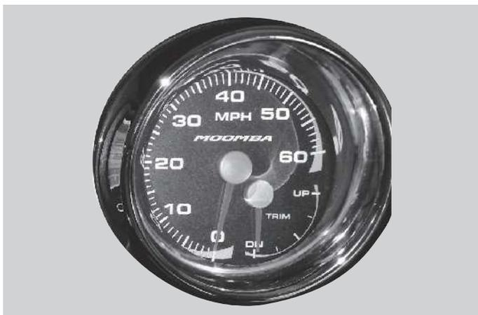
The speedometer indicates the water speed of the boat in miles per hour. It is recommended that the speedometer be checked for accuracy after each 100 engine hours.
