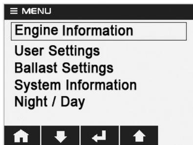
Utilize the Soft Keys to: • Go to the Home screen (Soft Key 1) • Move the cursor down to the next selection (Soft Key 2) • Enter the highlighted menu selection (Soft Key 3) • Move the cursor up to the previous selection (Soft Key 4).
