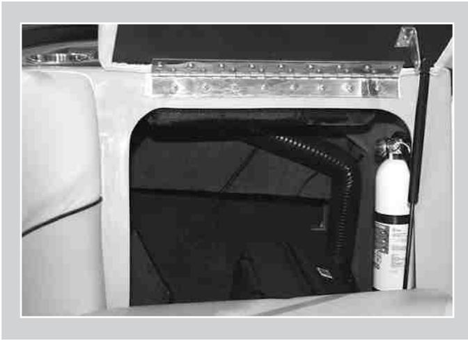
A standard Coast Guard approved fire extinguisher is provided on all Moomba boats. The fire extinguisher is located on the port side behind the observer's seatback.
