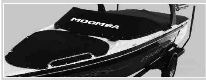
The optional cockpit cover is a snap down storage cover designed to help protect the interior of your boat. To install the cover, start at the windshield and work towards the transom. Be sure to install the cover poles to prevent water pocketing.
