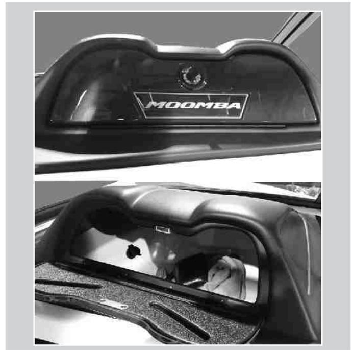
To open the glove box, press the black round cylinder down while lifting the black finger tab. Once open, the lid is supported by a spring.
