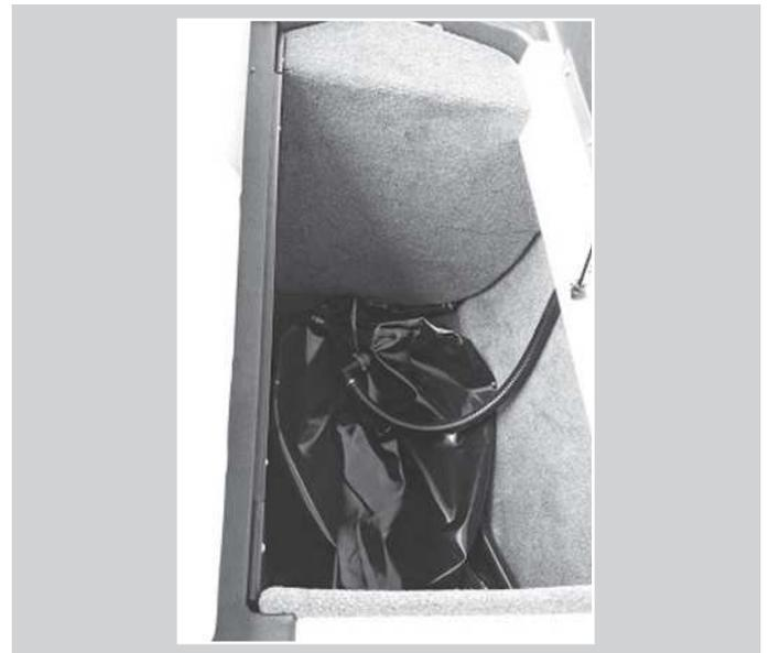
Care should be taken that the ballast bags are situated properly with the fill hose on top and drain hose on bottom and that all fittings are installed securely. The bags should not be twisted and the bags should be free to expand and drain completely. Care should be taken to prevent sharp objects from coming in contact with the bags. Cuts and punctures to the bags are not warrantable.
