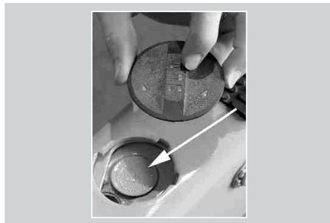
To check brake fluid, twist black cap and remove. Pry rubber plug out of reservoir. Follow instructions printed on plug. Use DOT 3 Brake Fluid.
