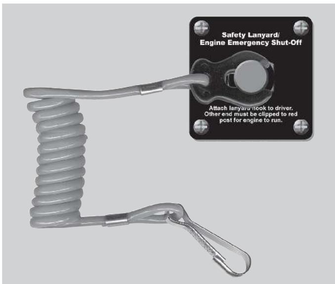
Your Moomba is equipped with a Safety Lanyard/Engine Shut-Off switch. In order for the engine to run, the plastic tip of the safety lanyard must be attached to the switch. If the clip is removed from the switch, the engine will not run.
