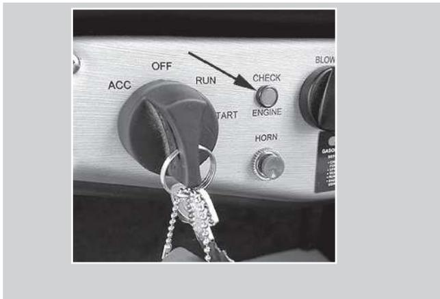
Your boat has an red check engine light. It functions much the same as the check engine light in your car. If the engine control module senses certain engine parameters out of range or a trouble code is set, the light will come on.
