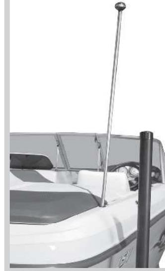
The removable pole light is stored in the bow. Always check for proper alignment when inserting the pole light into the receptacle.
