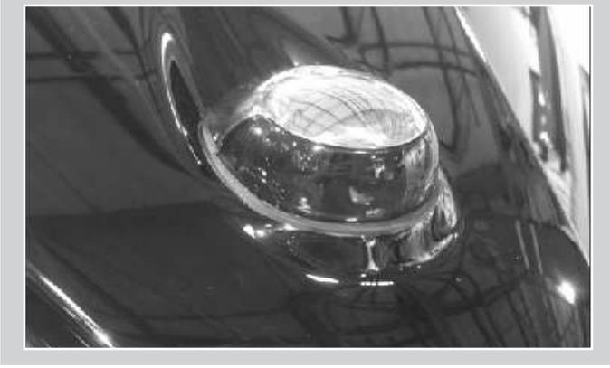
The bow light is located on the forward deck. To alert other boaters to your position and direction while underway at night, the light is green on the starboard side and red on the port side. To replace the bulb, remove Phillips screw to lift cover.
