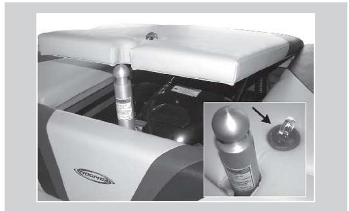
To access the engine compartment, turn latch and pull to raise the center sun deck lid. When the ski lockers and engine compartment lids are closed, the upholstered lids double as a cushioned sun deck.
