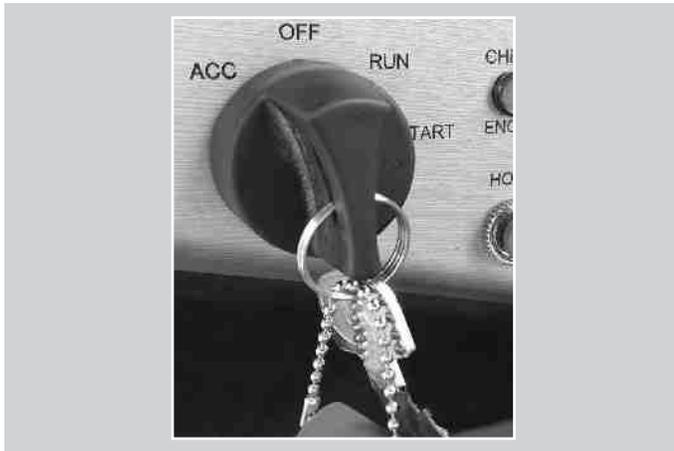
Two ignition keys are provided with the boat. Key entry into the ignition may sometimes be difficult due to the rubber boot protector. Please do not unduly force the key into the ignition. Key tumblers are located vertically, so the key should be vertical when placed into the switch.
